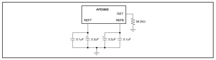
Figure 58. Suggested Decoupling on the Reference Pins
