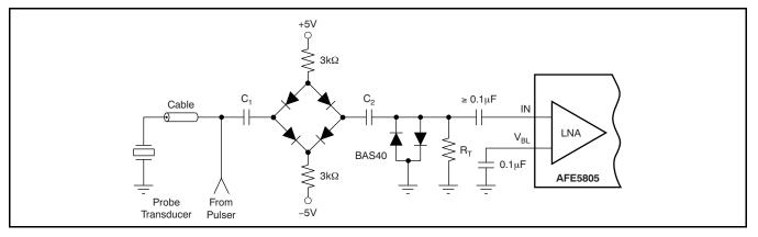
Figure 51. Typical Input Overload Protection Circuit of an Ultrasound System
