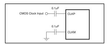
Figure 57. Single-Ended Clock Driving Circuit When DIFF\_CLK = 1
