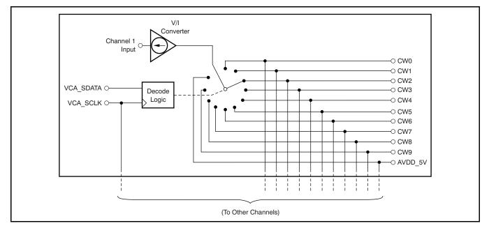
Figure 42. Basic CW Cross-Point Switch Matrix Configuration
