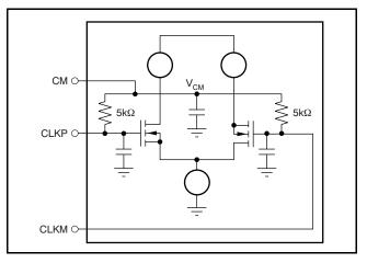
Figure 55. Internal Clock Buffer
