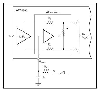
Figure 52. External Filtering of the V<sub>CNTL</sub> Input
