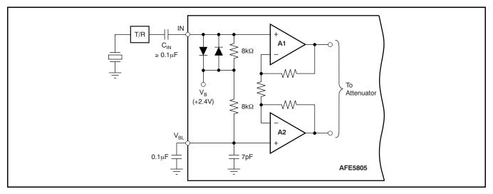
Figure 50. LNA Channel (Simplified Schematic)
