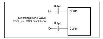
Figure 56. Differential Clock Driving Circuit (DIFF\_CLK = 1)
