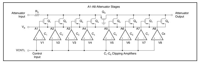
Figure 47. Voltage-Controlled Attenuator Simplified Schematic
