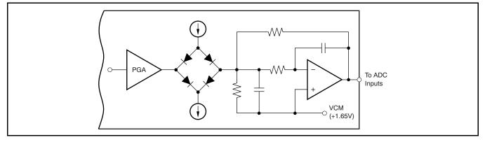
Figure 49. Clamping Stage and Low-Pass Filter (Simplified Schematic)
