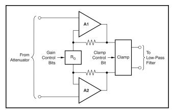
Figure 48. Post-Gain Amplifier (Simplified Schematic)
